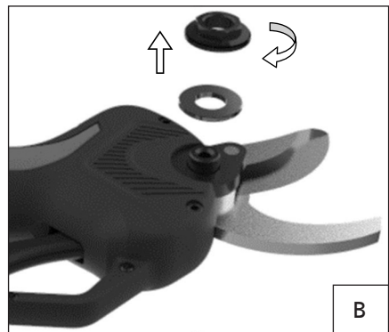
B. Remove the nut clockwise as shown and remove the flat needle roller bearing.
